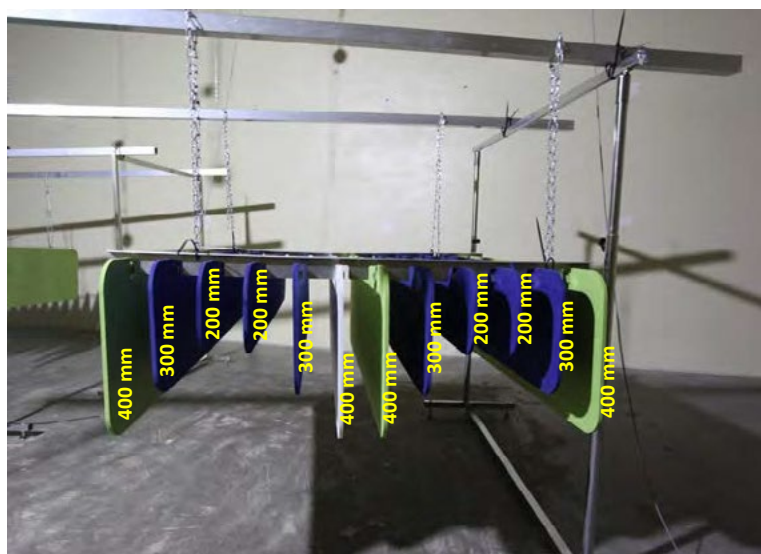
1 object = 1 baffle element with 12 blades in wave form
