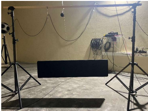
Photo: sample mounted in the reverberation room
