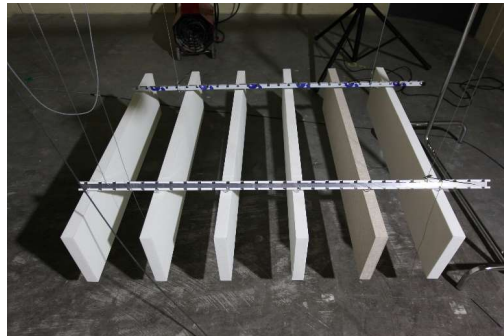
Photo Test n° 12 : one objet = 1 grid with 6 Slimbox Baffles suspended from U-shaped rails with 250 mm spacing between the centres (suspension points) of the baffles
