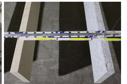
Photo Test n° 13 : one objet = 1 grille with 3 Slimbox Baffles suspended from U-shaped rails with 500 mm spacing between the centres (suspension points) of the baffles
