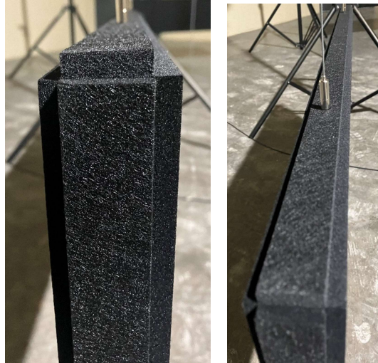
Photo: section view, Slimbox baffle
