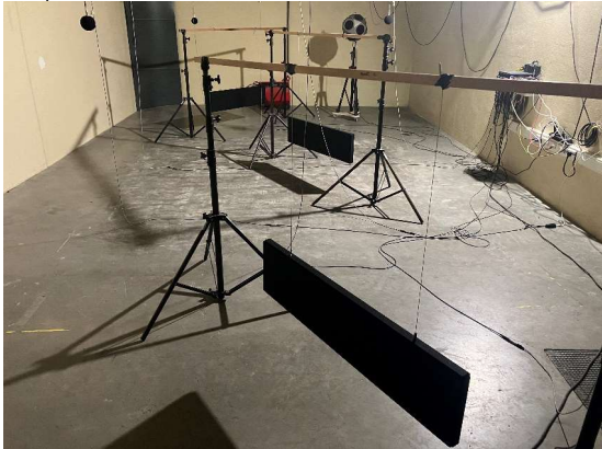
Photo : suspension height 300 mm
