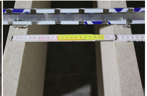
Photo Test n° 12 : one objet = 1 grid with 6 Slimbox Baffles suspended from U-shaped rails with 250 mm spacing between the centres (suspension points) of the baffles
