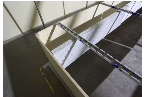
photo : detail of the SlimBox Baffle assembly during the test set-up.
