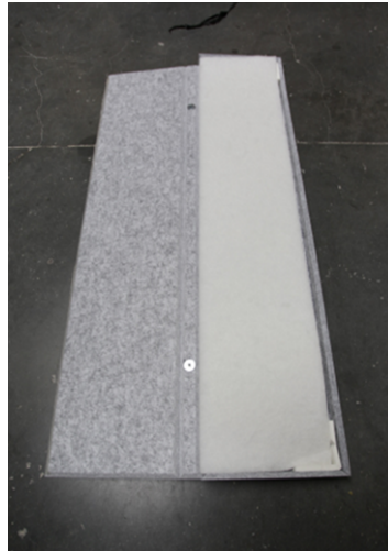
photo : Interior of SlimBox Baffle (1120 x 260 x 40 mm) with PE-wool (thickness \pm 22,5 mm)
