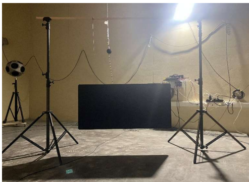
Photo: sample mounted in the reverberation room
