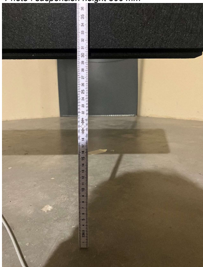
Photo : suspension height 300 mm
