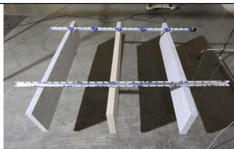
photo: Test n°13: 1 grille with 3 Slimbox Baffles
