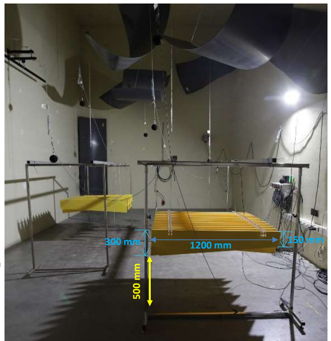
1 object = 1 baffle element with 12 alternating trapezium blades of 1200x(150/300) mm
