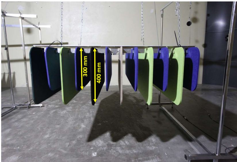
1 object = 1 baffle element with 12 alternating blades of 1200 x (400/300)mm
