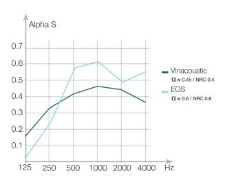
• The assembly with a simple plenum (without mineral wool) provides a highly effective acoustic solution: high absorption from low frequencies, very balanced curve throughout the spectrum
