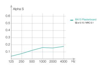
• The layer made of non-woven fibres is porous. Its thickness and the quality of the acrylic printing inks provide a modest absorption of medium to high frequencies
