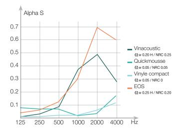
$\bullet$  To comply with the acoustic standards (NRA : New Acoustic Regulations) in communal areas with a concrete base : Vinacoustic  $\Omega$ w 0.20H or Eos  $\Omega$ w 0.25H  $^{\!\!\!(2)}$
