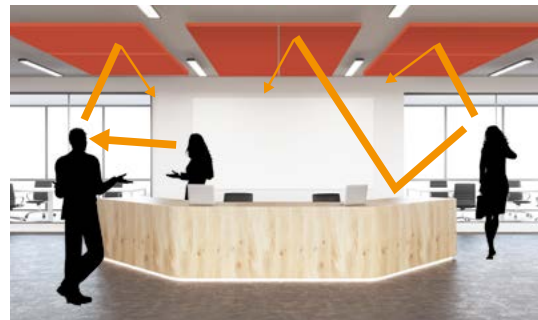
Fig B. With acoustic correction, the sounds are partially absorbed by the acoustic panels or wallcovering, improving comfort levels.
